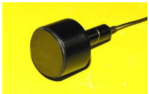
High temperature bismuth titanate ultrasonic transducer with THERMOCOAX coaxial cable
