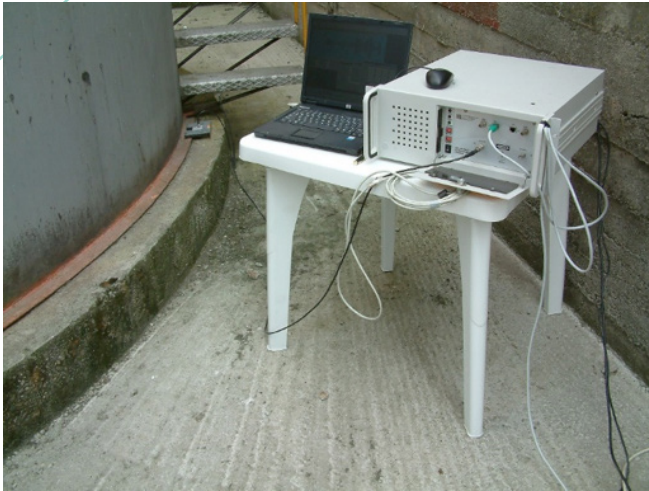
Experimental setup for the field tests of the tank with 8m diameter and partially filled with gasoline / diesel
