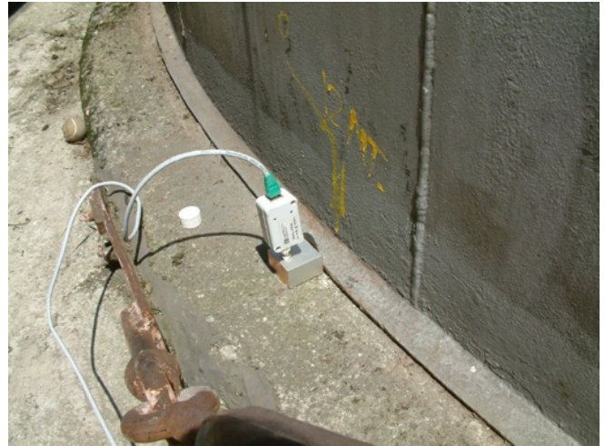
Experimental setup for the field tests of the tank with 8m diameter and partially filled with gasoline / diesel
