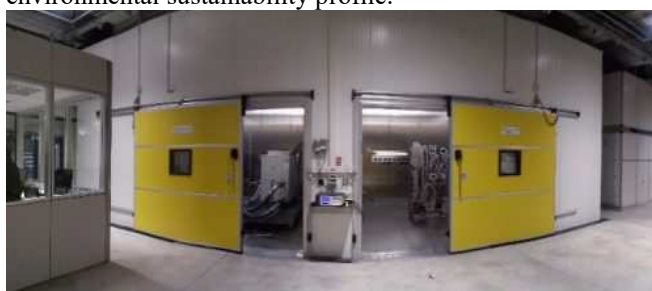
Fig. 6. PoliMi RELAB Double Chamber Calibrated Calorimeter
