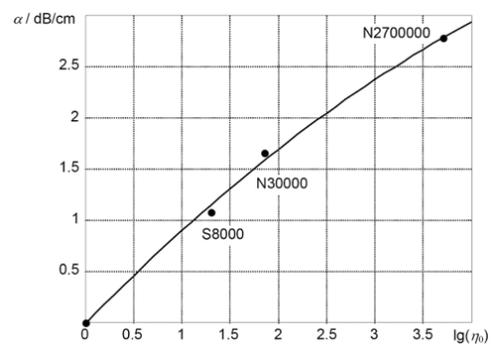
Attenuation coefficient  $\alpha$  of the SH0 wave in the aluminium wave-guide versus dynamic viscosity
