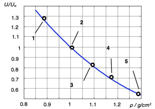
Dependence of the normalized amplitude  $U$  in the reflected signal on the density of loading liquid (1 -ethyl alcohol, 2 -distilled water, 3 -20% sugar/water, 4 -40% sugar/water, 5 -60% sugar/water)
