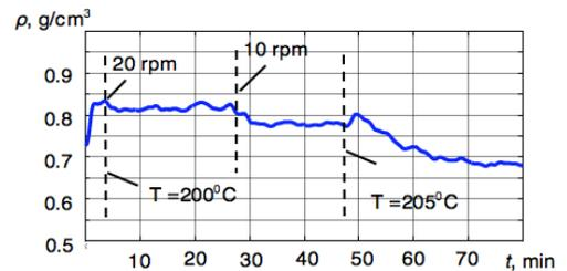
Variations of the density of the virgin PP melt for different temperatures and pressure (rpm -revolutions per minute)
